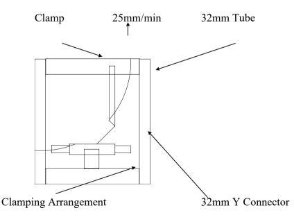
Prepare an assembly as above and using a suitable clamping arrangement secure the 32mm protective tube section to one of the tensometer jaws. Place the branch tube in the other jaw and perform a destructive test at a rate of extension of 25mm/minute.
